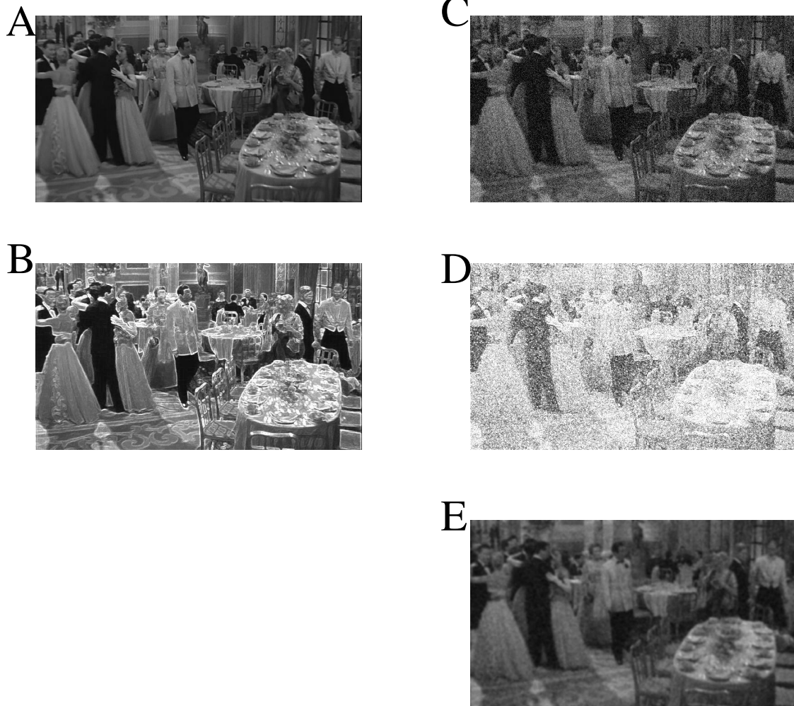
Figure 7.5: A) Original image. B) Edge enhanced version (high pass filtered). C). With noise added. D). The same edge enhancement does not gain anything. E). In this case low pass filtering works better. Note: made with GIMP for illustration purposes only, the filters were not exact.
