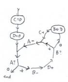
Here, for clarity, we have assumed given some very simple components. 'C=0' and 'D=0' do what they say; 'B  $\leftarrow$  D' copies the value of D to B, setting D to 0 in the process.
