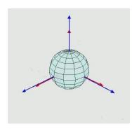
yaw-pitch-roll or Z-Y-X (3-2-1) --> used in flight!
