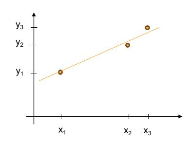
☐ Minimise the residual error between sample and line prediction:
