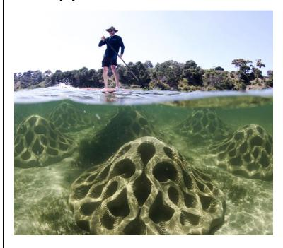
Built and deployed modular, diver-assembled reef lattices as experimental substrates to compare materials and attachment methods; to learn what forms/materials support colonization.
