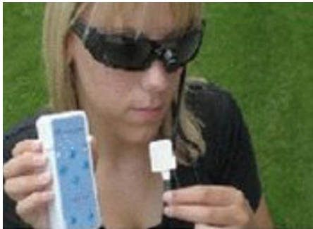
BrainPort V100 : a non-surgical assistive device that aids blind people in seeing with their tongue
