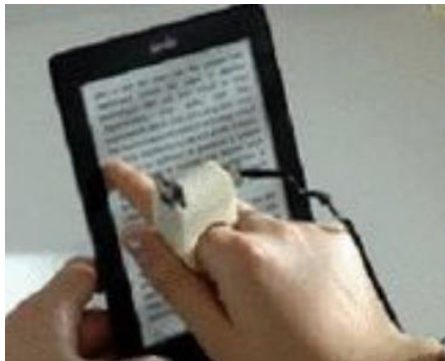
FingerReader : a small finger-worn form factor from the MIT Media Lab that assists blind users with reading printed text on the go
