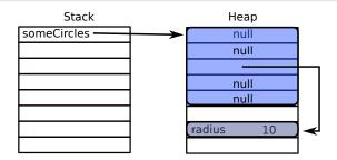
An array of objects is automatically initialised with null. To fill it, space for each object needs to be allocated explicitly.
