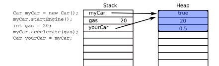
The memory of each object is put on the heap, while a reference to that object is kept on the stack.
