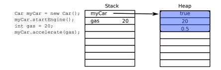
The memory of each object is put on the heap, while a reference to that object is kept on the stack.
