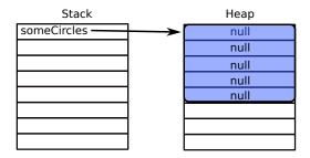
An array of objects is automatically initialised with null. To fill it, space for each object needs to be allocated explicitly.
