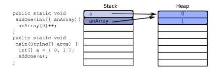
The array content on the heap is changed as a side effect of the function addOne.
