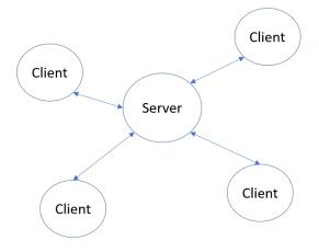
Client-server architecture: logical view for web-based and mobile software systems
