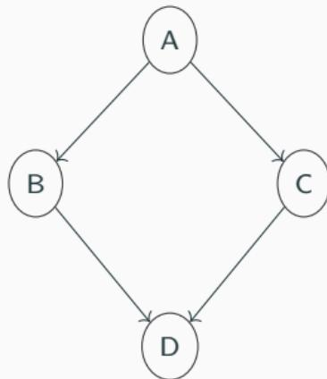
$$\begin{aligned} P(A|d) &= \alpha \sum_b \sum_c P(A, b, c, d) \\ &= \alpha P(A) \sum_b P(b|A) \sum_c P(c|A) P(d|b, c) \end{aligned}$$
