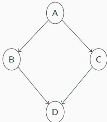
$$\begin{aligned}P(A|d) &= \alpha \sum_b \sum_c P(A, b, c, d) \\&= \alpha P(A) \sum_b P(b|A) \sum_c P(c|A) P(d|b, c) \\&= \alpha f_1(A) \sum_b f_2(B, A) \sum_c f_3(C, A) f_4(B, C)\end{aligned}$$
