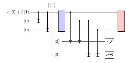
where the first measurement is a computational basis measurement of  $Z_1 \otimes Z_2$ , and the second measurement is a computational measurement of  $Z_2 \otimes Z_3$ . The blue box is hiding a (possible) error that has occurred, which will be nothing (identity) or a bit-flip error X that acts on any one of the three qubits. The pink box is hiding the corresponding correction.
