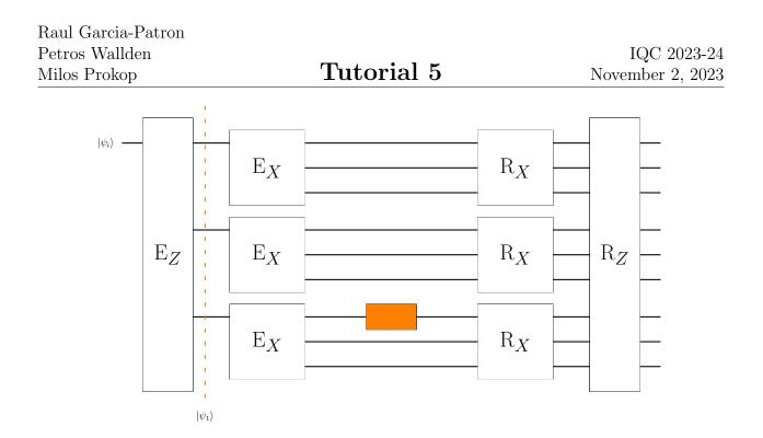
where  $E_Z$  and  $E_X$  are the encoding circuits, and  $R_X$  and  $R_Z$  are the recovery circuits. The orange box in the circuit signifies a single qubit error occuring on the 7<sup>th</sup> qubit. Assuming that the initial state is  $|\psi_i\rangle = a |0\rangle + b |1\rangle$ ,
