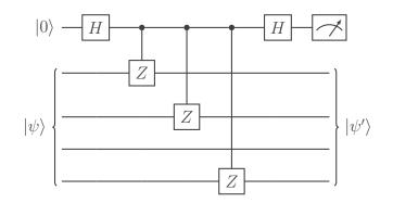
Now we can insert double Hadamard gates in between controlled-Z gates, as they are equivalent to identity:
