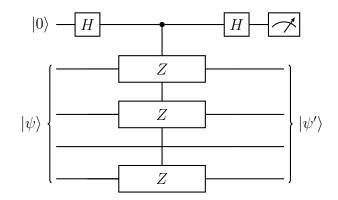
**a.** Derive the action of the three-qubit parity operator  $P = Z \otimes Z \otimes I \otimes Z$  on the computational basis state  $|x_1x_2x_3x_4\rangle$ . What are the eigenvalues of the operator P?
