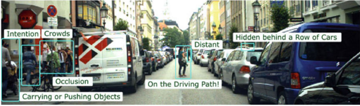
Figure 2: Typical challenges to pedestrian detection for automated driving.
