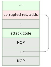
The exact address of the attack code in the stack is hard to guess. The attacker can increase the chance of success by allowing a range of addresses to work. The overflow uses a *NOP sled*, which the CPU execution "lands on", before being directed to the attack code.
