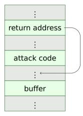
The malicious argument overwrites all of the space allocated for the buffer, all the way to the return address location. The return address is altered to point back into the stack, somewhere before the attack code. Typically, the attack code executes a shell.
