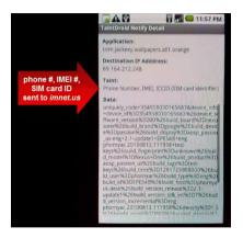
Taintdroid uses a modification of the Android framework to track data flows at runtime. See the **demo video**.
