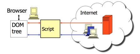
A programming approach might ensure confidentiality or integrity, by making sure that scripts do not mix data from different domains.
